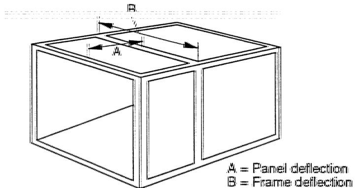
**Figure 2 — Illustration of panel and frame spans of air handling units**
