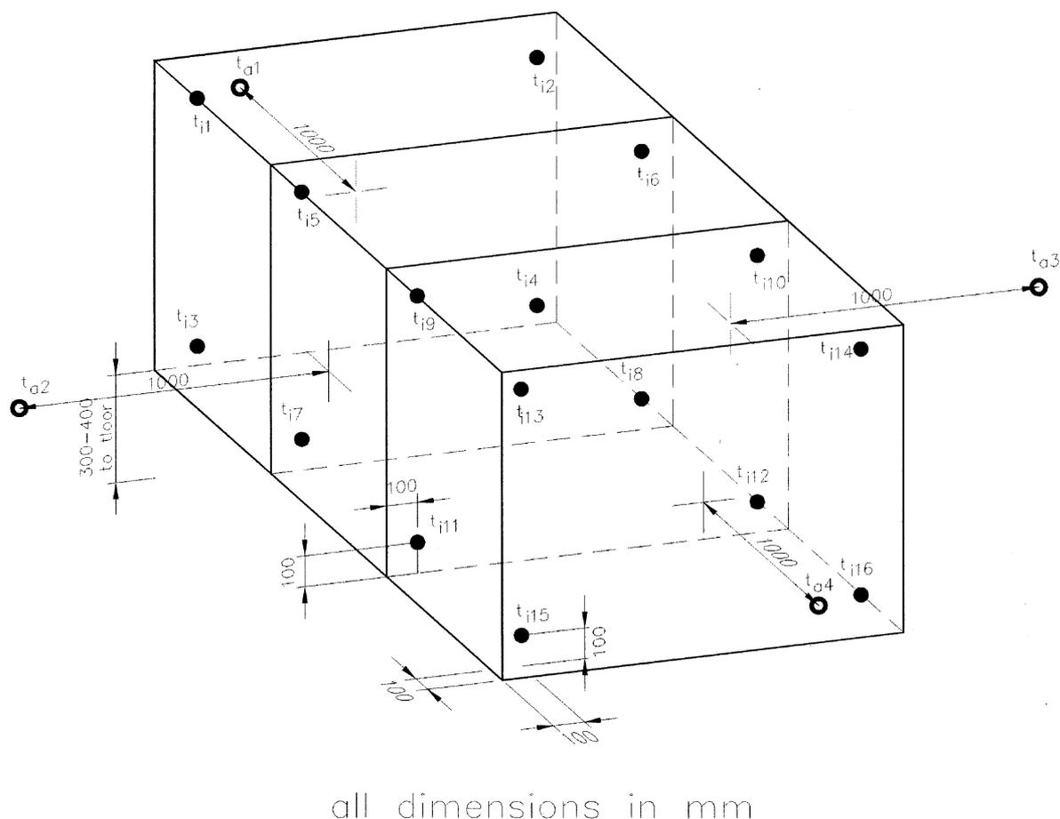
**Figure 10—Zoning and installation of measuring devices**
